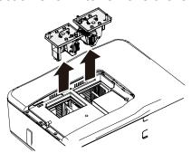
4. Install the new lamp module(s) and replace the lamp cover.
