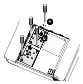
3. Pull firmly on the module handle in the direction shown to remove the lamp.
