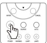
Press the POWER button again on the OSD control panel or remote control to confirm power off. The cooling fans continue to operate and the power LED flashes orange. The cooling fans stop operating when the projector turns off.
