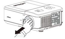
2. Make sure the lens is pushed into the holder and turn it clockwise to the "Lock" position. When turning the lens, the "Click" sounds twice to indicate that the lens is completely fixed.
