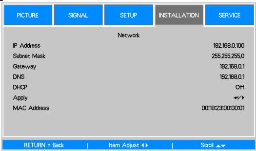
Use this function to set up network configurations so that you can control the projector via the network.
