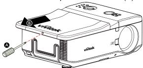
2. Loosen the two captive screws on the lamp module (A). Lift the module handle up as shown (B).
