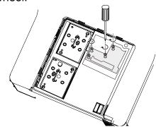
3. Lift the color wheel in the direction 3. Place the color wheel (A) and tighten the screw on the lamp cover as below illustration (B).
