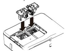
5. Tighten the two captive screws on the lamp module.
