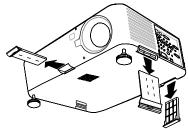
4. Lift the filter foams from all three filter holders in the direction shown.Remove them completely from each filter holder and discard.
