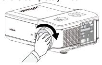
Check if the lens is fixed successfully by pulling the lens out of the holder gently.
