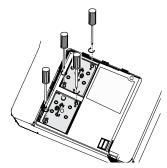
6. Place the lamp cover and tighten one screw on the cover as below illustration.
