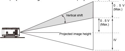
The projected image can be moved down by 50% (0.5V) if the project is installed via a ceiling mount.
