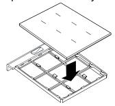
6. Replace the filter holders by pushing gently in the direction shown on below illustration.
